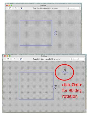
Then place it where you'd like it to be. If you'd like to rotate, press **Ctrl-r** until the correct direction. You can escape the component cursor mode by pressing **esc** key.
