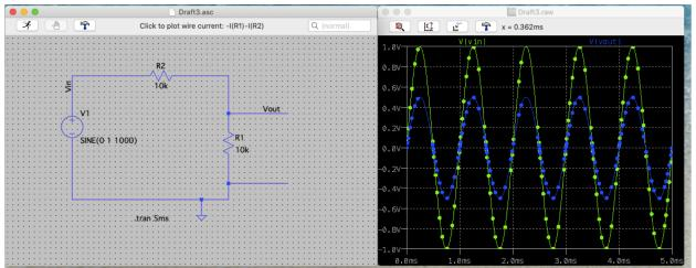
\*\* If you click while holding down Shift-Ctrl, the voltage probe will change to the **current probe cursor** and clicking will make current vs time plot appear (on current values showns on right y-axis).
