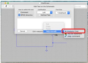
14. We will mostly use **transient** and AC analysis. **Transient** is for time-domain (i.e. x-axis is time as oscilloscope screen).
