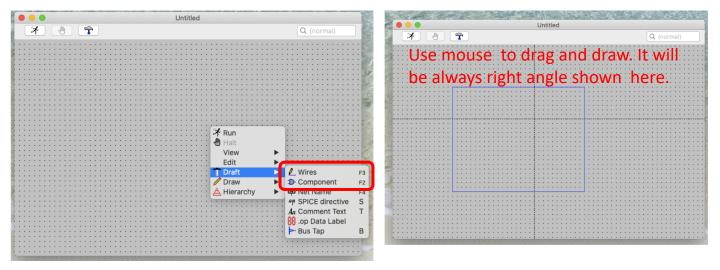
6. Now add resistor(s) (or other parts). Again go to **Draft>Component type Resistor**
